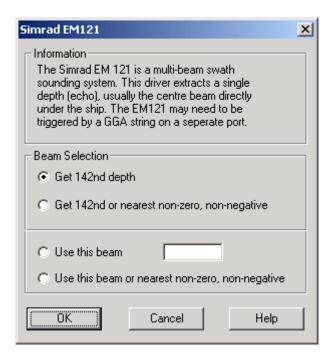
In the Beam Selection sections you can instruct WinFrog to accept the depth reading from either the 142<sup>nd</sup> beam (which is typically directly beneath the ship) or to accept the depth from either the 142<sup>nd</sup> beam or the nearest beam that does not return a zero or negative number. You can also specify a particular beam (by entering the number) for WinFrog to take the depth from or the beam nearest to the specified beam that does not return a zero or negative number.
